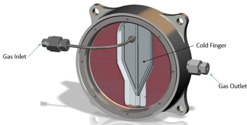
Figure 1 - The Water Droplet Demonstration Chamber (VDU Design)
